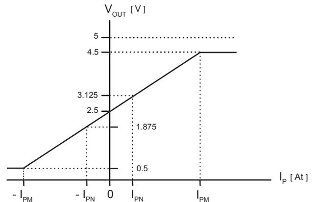
**Note:** <sup>1)</sup> Output voltage when LTSR 25-NP is used with internal reference.
